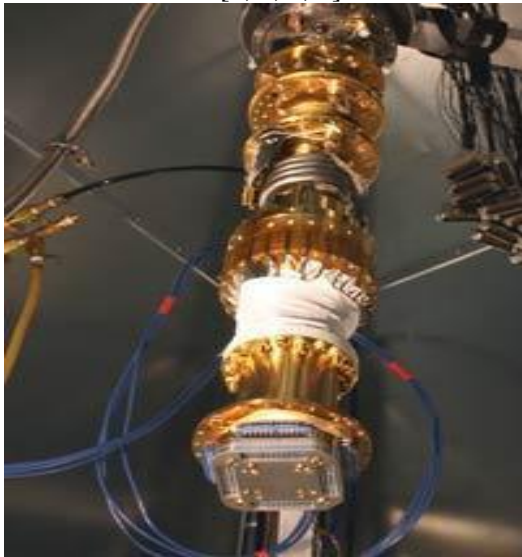
Figure 2: D-Wave's 16-qubit quantum computer [2].
